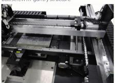
由精密滚珠丝杆+运输导轨构成的XY龙门,更加灵活的作业方式,有效作业区域400\*400mm。 The XY gantry composed of precision ball screw + transportation guide, more flexible operation mode, effective operation area 400\*400mm
